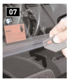
The alarm module should be fitted behind the glovebox, which means you'll need to remove it. We've been here before but in case you weren't paying attention, start by removing the two screws in the outer top corners of the dash vents.
