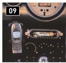
First job is to get the factory radio out. Start by removing the four screws at the top of the two silver upright struts.
