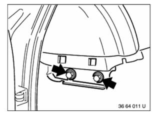
Remove left and right screws and remove dashboard.
