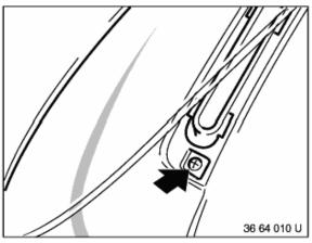
Unclip frames for left and right defroster nozzles. Remove outer screws on left and right.
