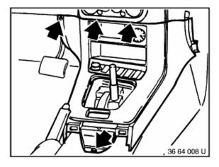
Remove screws and remove centre console.
