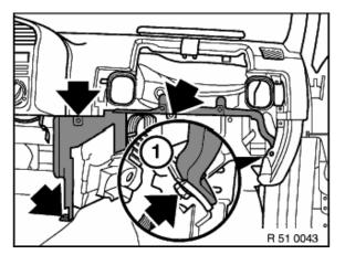
Only with passenger airbag: Unfasten screws and remove rod (1).
