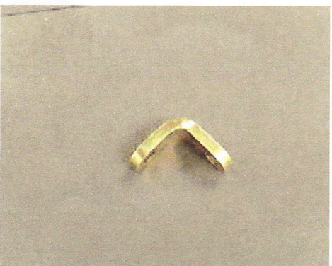
B0-0010, AFPR Mounting Bracket - Mounts the AFPR to the front of the engine. ✓
