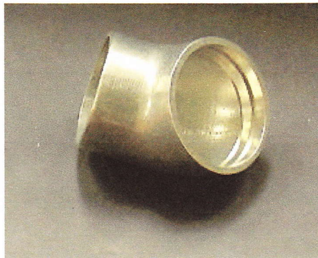
B0-0015, Small Intake Elbow - Connects the bellows with the AFM. ✓
